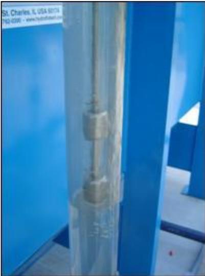
**NOTE:** The level sensors **MUST** be maintained clean. If allowed to foul and malfunction the RAD pressure vessel will fill with water and bubbles will **NOT** be created. They are easy to remove and clean while the RAD is operating by closing the isolation valves and venting pressure with the sight tube drain valve.
