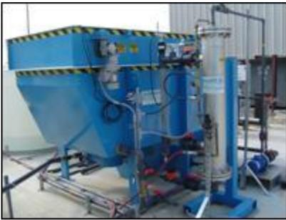
A DAF (Dissolved Air Flotation) system creates microscopic air bubbles that are attached to incoming wastewater particles in order to float them. Once floated, they are separated from the wastewater and skimmed from the top and into the float scum chamber. The treated wastewater then exits from near the bottom of the DAF. The DAF creates its air bubbles with a sub-system called a RAD (Recycle Air Dissolving) system. Proper operation of the RAD system is key to DAF performance.
