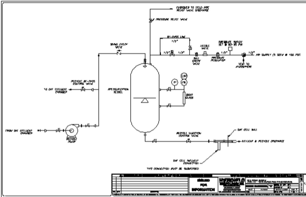
It is recommended that the RAD pump be allowed to operate continuously in order to maintain the float blanket in the DAF. If the RAD system is shut down the float blanket will degrade and floated material may sink and be flushed out with the effluent during the next startup.
